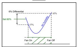
Fan on when air humidity 3% below set point. Fan off when air humidity 3% above set point. To ignore humidity set to 99%
