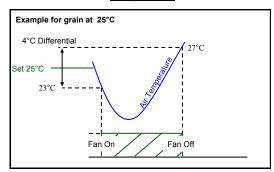
Fan on when air temperature 2°C below set point. Fan off when air temperature 2°C above set point. To ignore temperature set to 99°C
