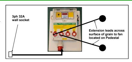
Recommended electrical and socket requirements for connection of a board-mounted controller to Pile-Dry Pedestal Fans is as follows:
