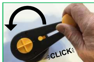
Rotate handle anti-clockwise until it clicks a few times
