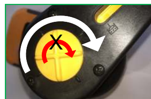
Ensure the yellow + remains stationary during grinding
