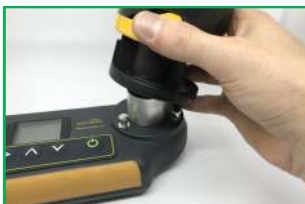
Place the Grinder-Compressor over the Grain Cup
