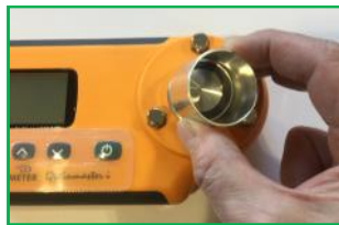
Place the Grain Cup on the Grain Cell
