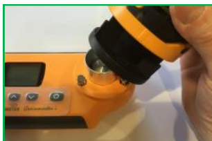
Place the Grinder-Compressor over the Grain Cup
