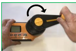
Rotate handle clockwise until there is no grinding noise
