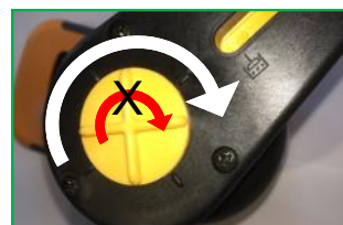
Ensure the yellow + remains stationary during grinding
