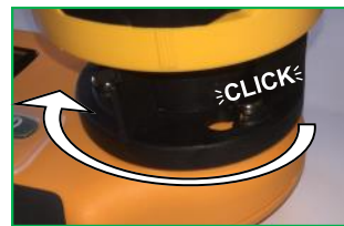
Lock in place by twisting clockwise against the lugs
