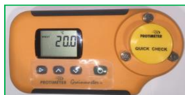
Press A or V to display Grain Cell temperature
