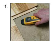
Use a Protimeter MMS or Protimeter Surveymaster in search mode to establish the area(s) of greatest concern on the sub floor.
