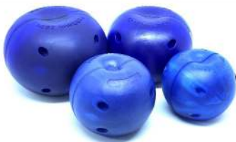
9 different apple shapes with many different weights have been created, to reflect different varieties and densities - allowing the shape to float at the same level as the real fruit
