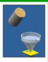
Hold the funnel spout level with the top of the cylinder, slide away the plastic insert and allow the cylinder to fill with grain.
