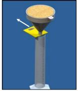
Using the plastic card, slide off any excess grain to leave a level top. Do not tap the cylinder or consolidate the grain in any way.
