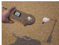
Grain Temperature Probe Fast response 1.5m probe to check stored grain temperatures.
