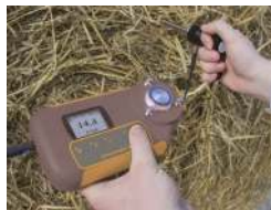
Bale Moisture Probe 600mm probe to check hay and straw bale moistures.
