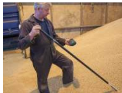
Moisture and Temperature Probe 1.5m probe to measure moisture and temperature of grain in the store.
