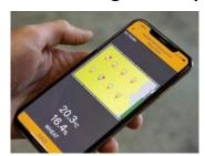
Download moisture and temperature readings instantly using the Grainmaster App. Readings from the meter or any of the optional probes can be sent instantly via Bluetooth to a smartphone, speeding up the recording process and making it easier to provide evidence for crop assurance schemes.
