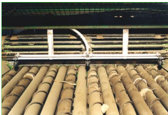
Harvester Mister 1 metre spray boom in position over dolmen rollers
