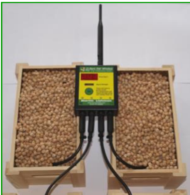
4-way Barn Owl Wireless Transmitter attached to cable sensors
