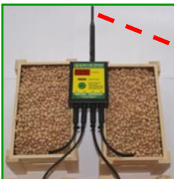
4-way Barn Owl Wireless Transmitter attached to cable sensors
