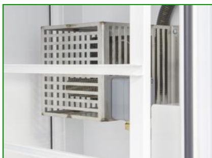
Interior of the 750 tuber Hot Box showing the fan, heater and humidifier
