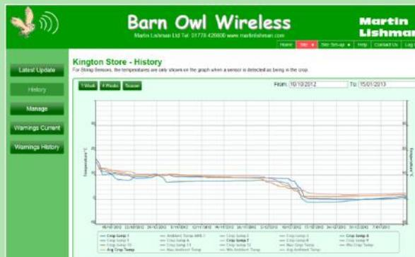
Typical example of cooling with FloorVent - the grain was cooled to around 10°C by the second week of October
