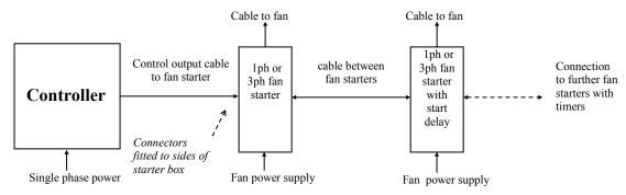
The actual location and arrangement of the components will depend on the existing electrical set-up in the building, and should be agreed between the purchaser and an electrician. Some typical arrangements are as follows:
