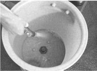
With a spray nozzle, thoroughly rinse the underside of the aeration disk until any visible biofilm or residue is removed. Then, use a non-abrasive sponge to thoroughly clean the surface of the tank fitting. Wipe dry the aeration disk and the area around the tank fitting before replacing the aeration disk.
