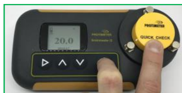
While the reading is visible, press A or V , the display will then show 0.0 , press Q to display Grain Cell temperature
