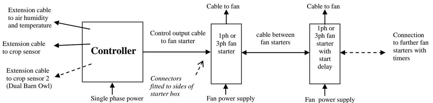
The actual location and arrangement of the components will depend on the existing electrical set-up in the building, and should be agreed between the purchaser and an electrician. Some typical arrangements are as follows:
